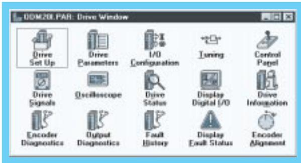
With just a click, the drive can be configured for a wide variety of operational modes (torque, velocity, position, step/dir, follower, etc.) Communications parameters may be set for single or multi-drop operation.
