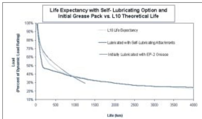
This chart illustrates how using the self-lubricating option, which combines the self-lubricating attachments and initial grease pack, will enable the bearing to achieve the L10 life expectancy under all loading condition. Note that for travel lives exceeding 30,000 km, recharging or replacing of the self-lubricating polymer is recommended.
