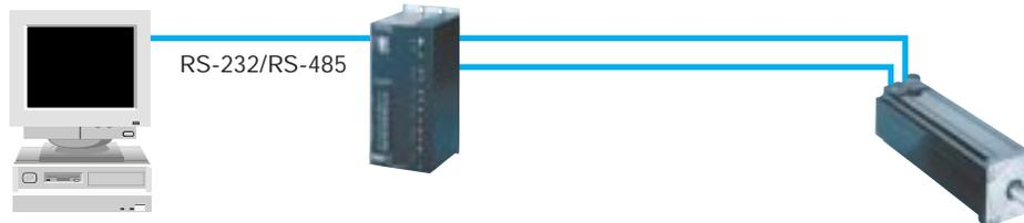
In general, an AXI-PAK without indexing is used when a separate servo or stepper controller (such as the TMC-2000) is utilized. The indexing option is required to give the AXI-PAK basic stand alone positioning capabilities.
